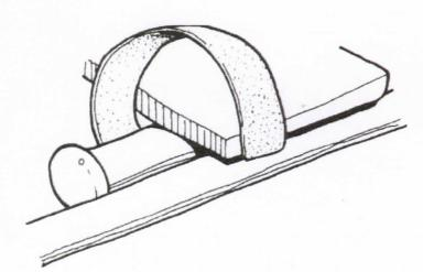
Place the linking apparatus (with the Velcro strap undone) on top of the bar to which it is going to be attached. Never attach from below the bar.
