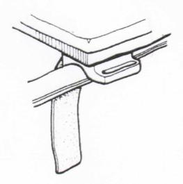
Place the pad/plank over the trestle bar. Ensure the bar is resting in the groove of the saddle bracket and the Velcro straps are loose.
