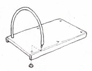
Insert the bolt on one end of the hoop into a fixing hole on the top of the bench/top. Secure from below with the retaining nut.
